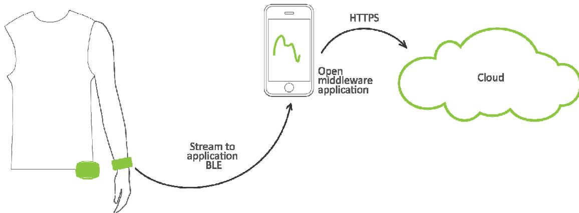
**Figure 3 Communication Methods of the Open middleware**
